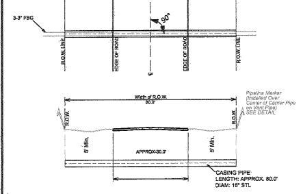
a: Vent Pipe to be installed on each end of casing. Minimum of 2' above natural ground.
